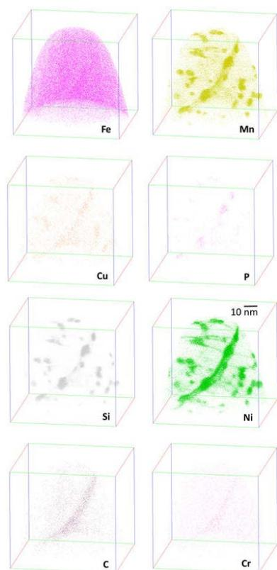
Atom Probe Tomography analysis of an ion-irradiated steel. APT images show a distribution of irradiation-induced Ni-Mn-Si clusters, P clusters, solute segregation to irradiation-induced dislocations and solute segregation to a grain boundary.
