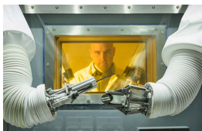
Operator and manipulator arms as seen from inside the hot cell
