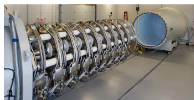
The Neutron Therapeutics proton accelerator will be used for the generation of the neutrons
